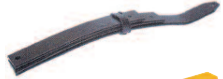
Front Heavy Duty, E-Z-Go Med/TXT 94-00 OEM: 70422G01; 70311G01; 70431G01; 75366G01. Item # SPN-1002
